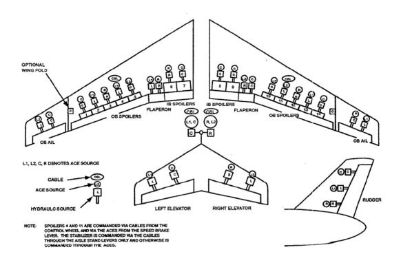
Figure 2. Primary Flight Controls Hydraulic/ACE distribution
