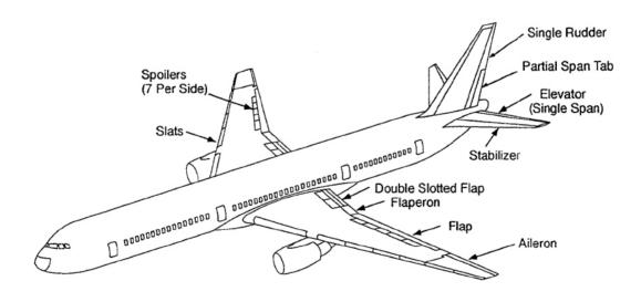
Figure 1. Primary Flight Control Surfaces.
